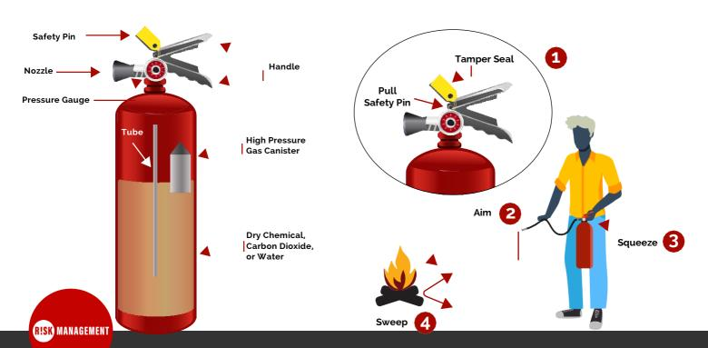
When it is time to use the extinguisher on a fire, remember PASS
